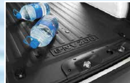
Plastic floor protection and trunk entry guard (43, 11)
